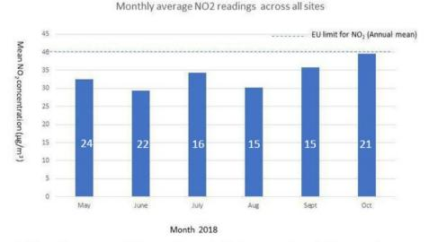
Figure 8: Monthly average NO<sub>2</sub> readings of all sites combined. The number on each bar shows how many locations data were received for.
