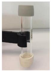
Figure 2: Diffusion tube used to measure NO<sub>2</sub>
