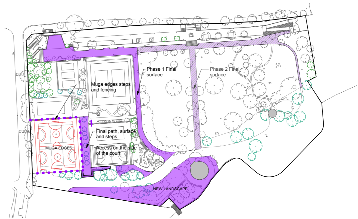
PHASE 4 Masterplan work : New paths surface and steps - Interface with LLAU work Edging of MUGA - South landscape
