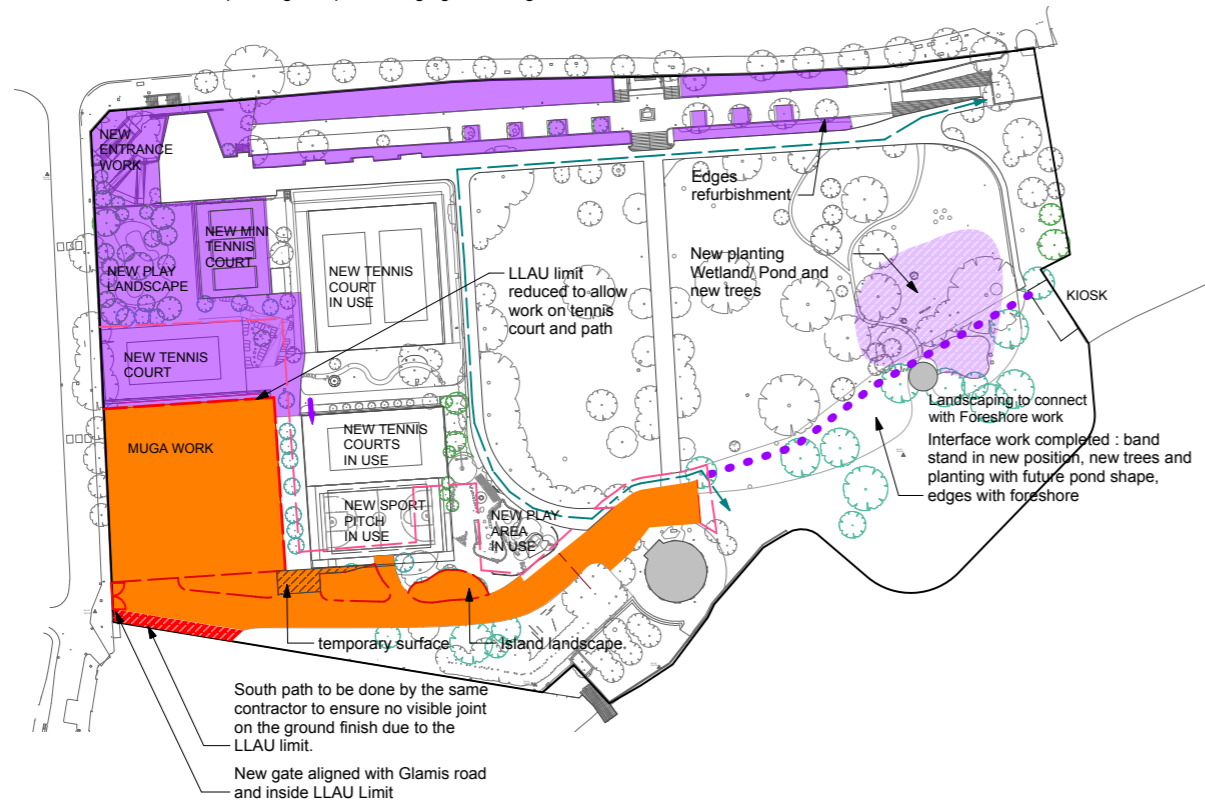
PHASE 3: Tideway on site : Muga, entrance and landscape works excluding steps and ramp Masterplan work : New North-West entrance - New play landscape and tennis court - Pond and wetland planting - Repairs / Edging / Planting
