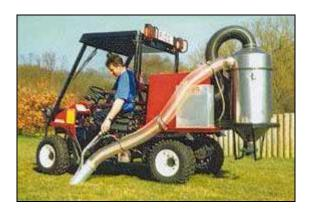
The collection unit contains its own engine, which drives a powerful vacuum unit capable of collecting 120 litres of all types of dog faeces. Once collected into a stainless steel container, it is mixed with disinfectant and water, which turns into slurry, leaving it pourable for disposal. A disinfectant spray pump is also fitted, not only to ease removal of stubborn faeces, but also to wash and disinfect the offending areas helping to protect children from toxcara canis.
