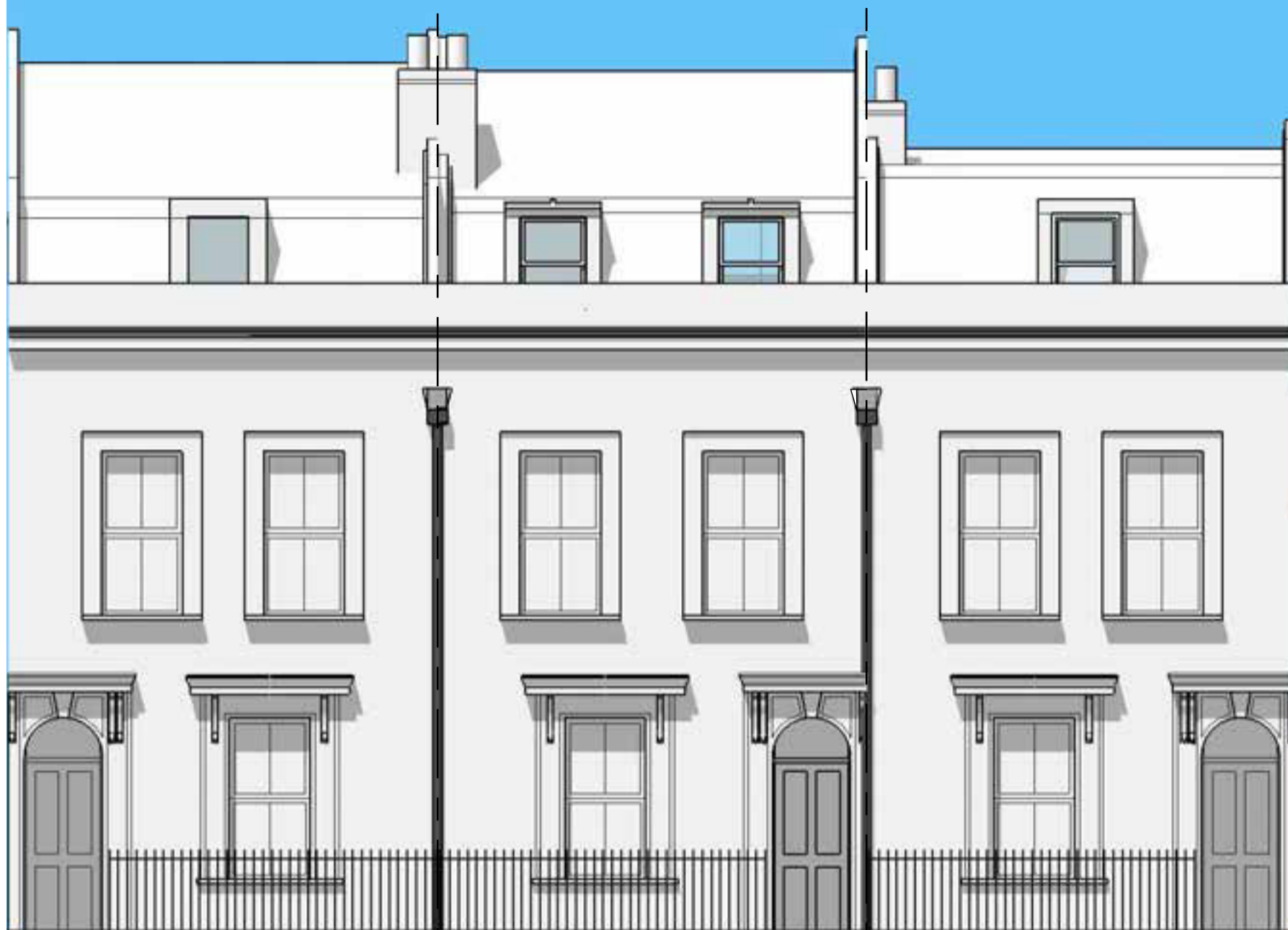
Option 1 Double pitch mansard, single dormer
