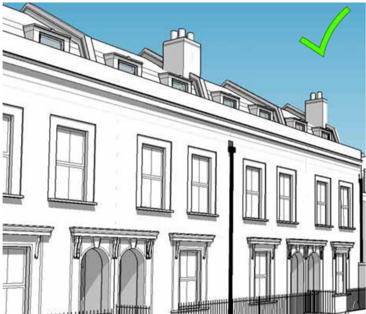
Mansard with larger set-back behind parapet wall
