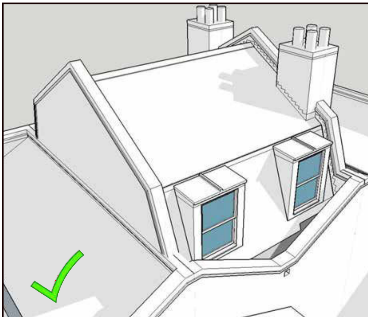
A dormer window to provide head height in a stairwell
