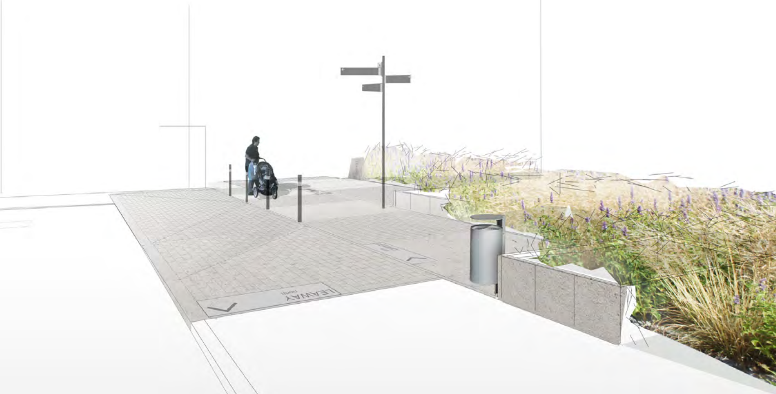
^ Incorporating all street furniture into coherent layouts on paving mats
