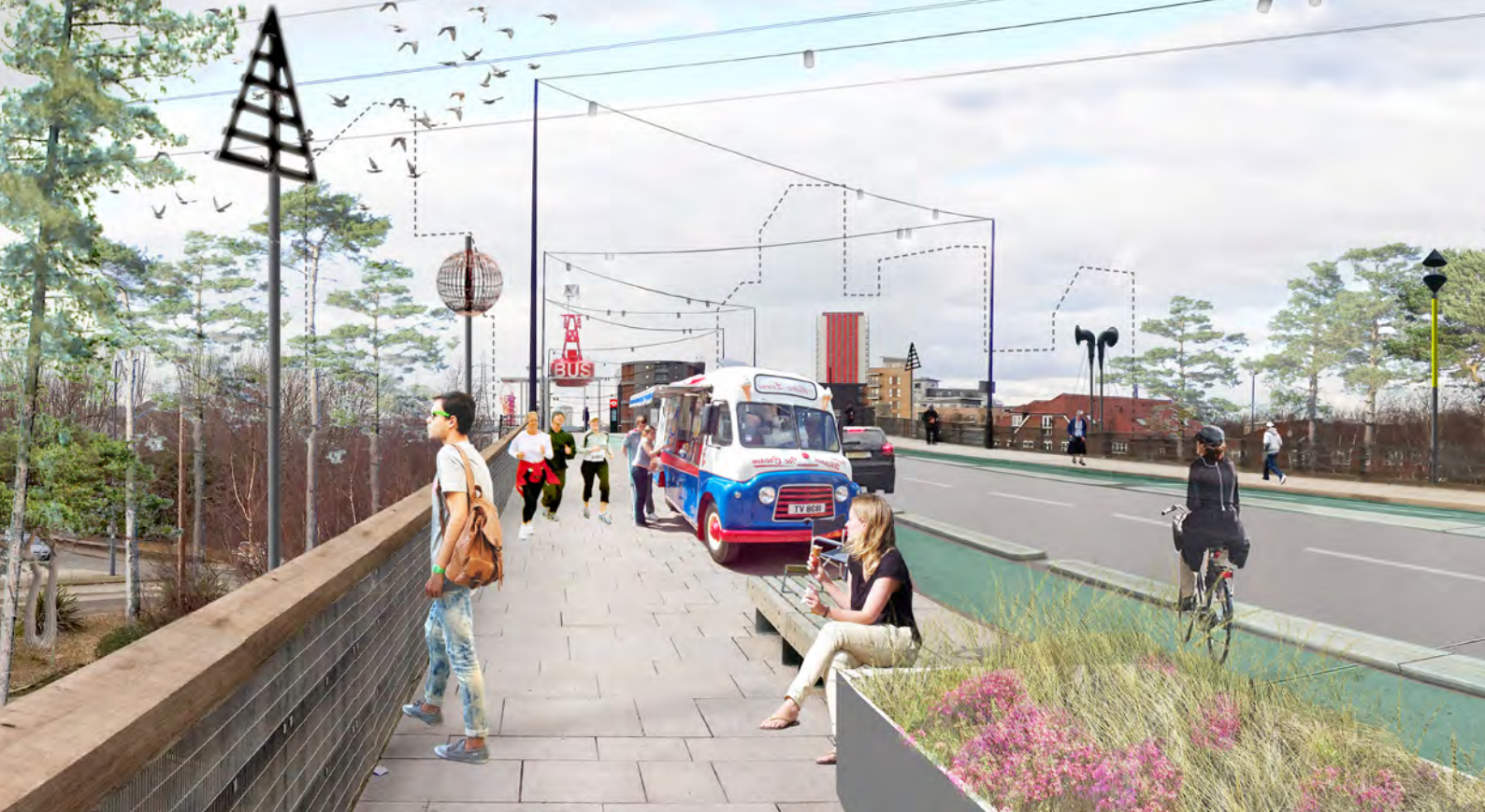
Visualisation of a re-surfaced viaduct, reducing carriageway widths to calm traffic, introducing segregated cycle paths and encouraging pedestrians to pause and enjoy the elevated views of the Royal Docks, Thames, Lea Valley and back towards the City of London.
