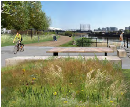
Cody Wilds, pre-cast concrete channels can be used both as a retaining edge and a bench.
