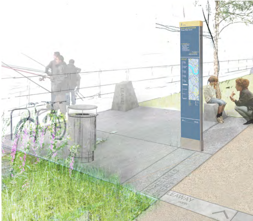
A Legible London Midilith as one of the street furniture elements that are consolidated on a typical paving mat
