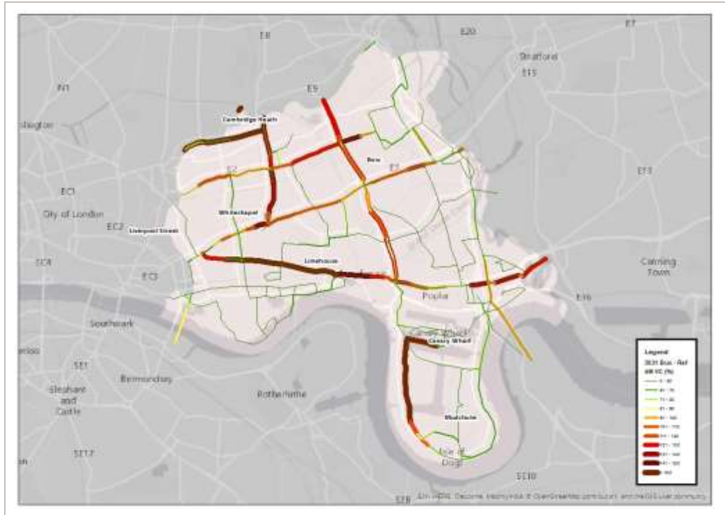
Figure 5.50 AM Peak Bus Patronage over Service Capacities (High Growth, 2031)
