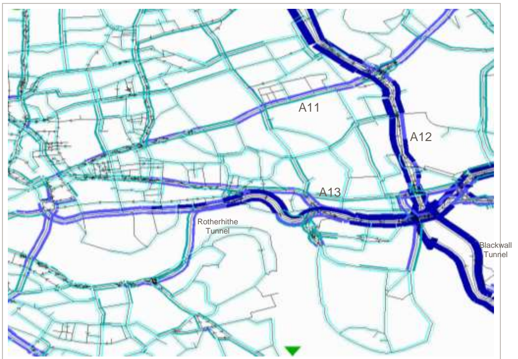
Figure 5.16 PM Peak Vehicle Flows (Central Case, 2031)
