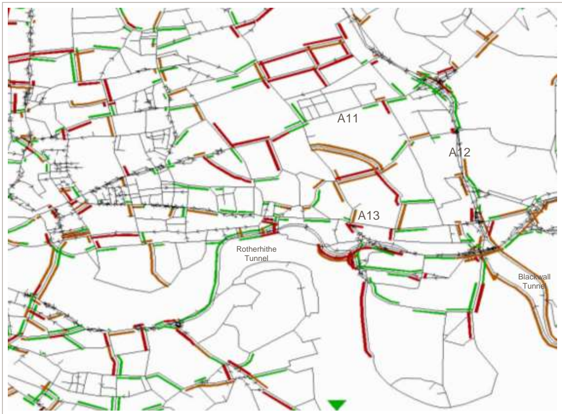
Figure 5.21 AM Peak Vehicle Volume over Link Capacity (Central Case, 2031)
