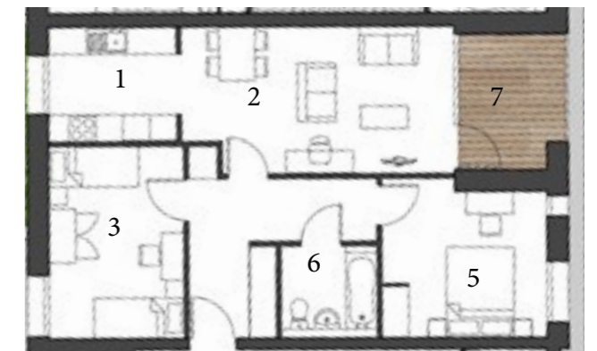
Example of dual-aspect floor plan including inset balcony (7); separation between kitchen (1) and living room (2) if needed, with possibility of cross ventilation through both; flexible twin room (5) which could also be used as a double bedroom; storage space integrated into plan. (image ©Levitt Bernstein)
