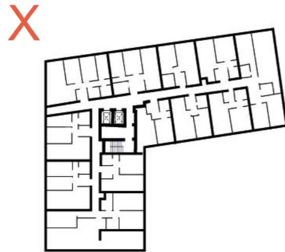
Corridors are long and angled so there is no visibility from one end to another.
