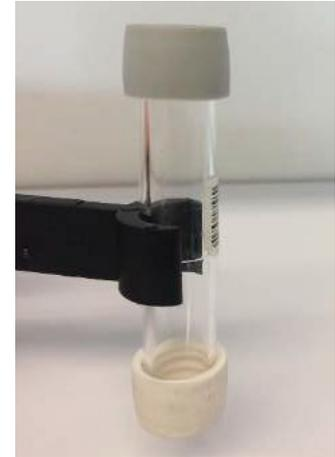
**Figure 2: Diffusion tube used to measure NO<sub>2</sub>**
