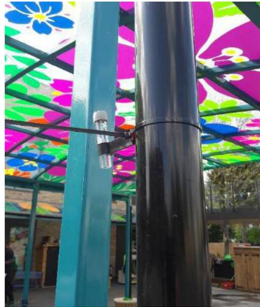
**Figure 4. Monitoring sites hosting diffusion tubes to monitor nitrogen dioxide**
