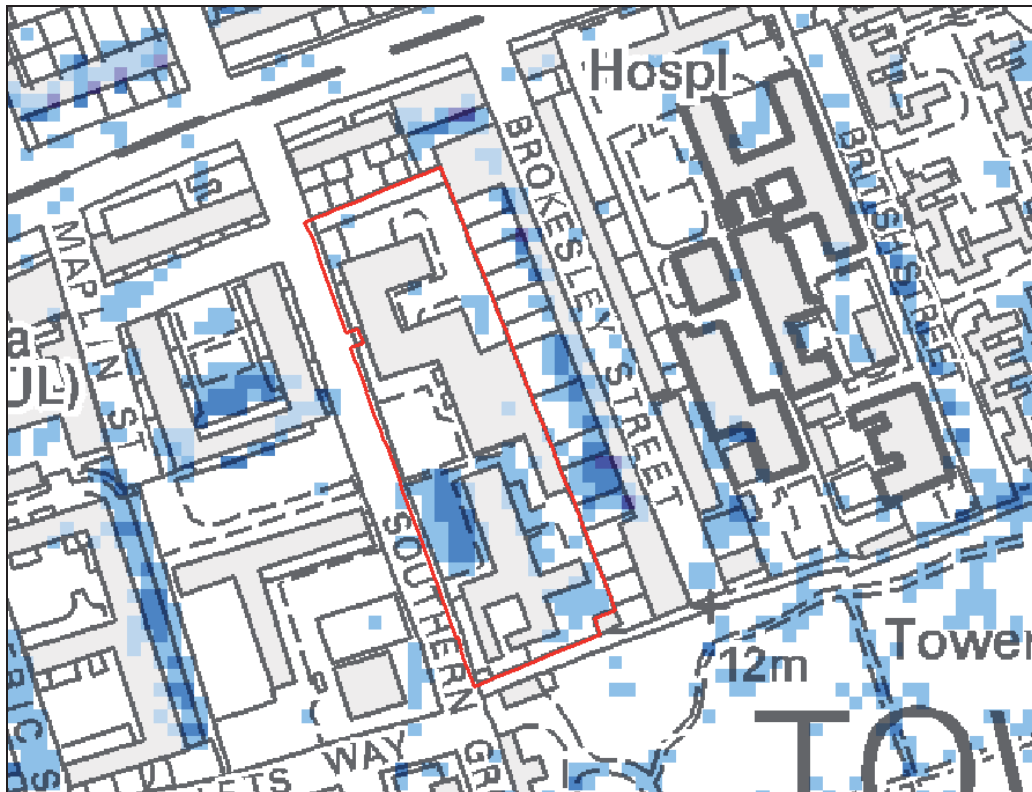
Figure 12-2 Maximum Depth of Surface Water in a 1% AEP Rainfall Event at the Southern Grove Lodge Site
