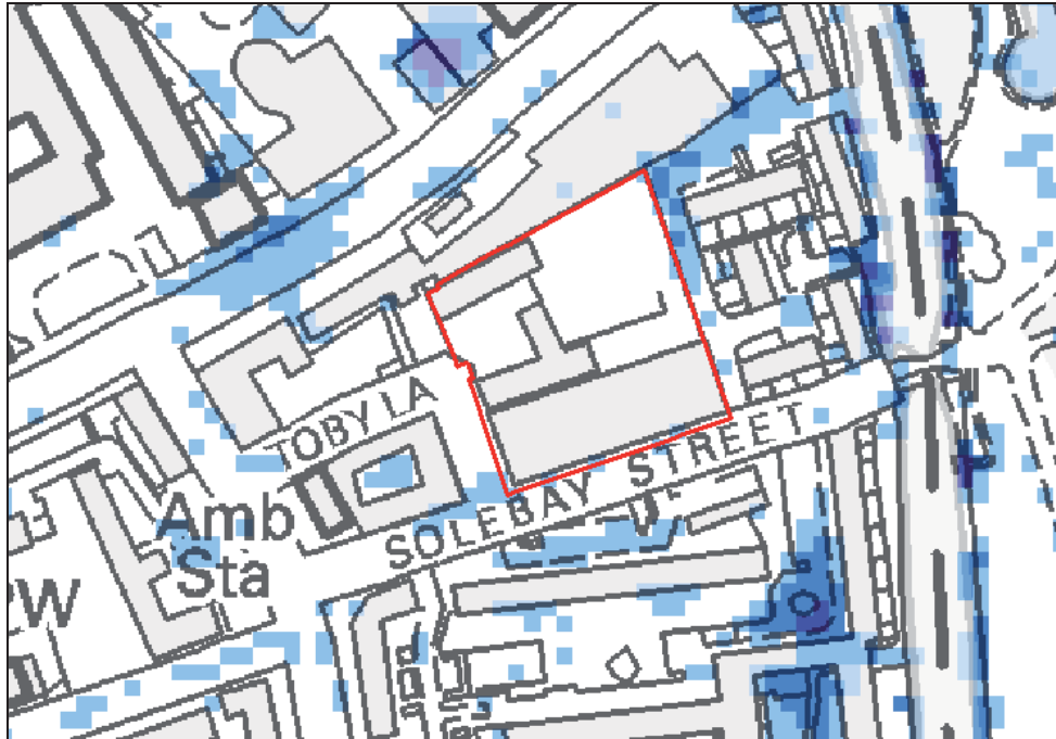
Figure 13-2 Maximum Depth of Surface Water in a 1% AEP Rainfall Event at the Toby Lane Depot Site
