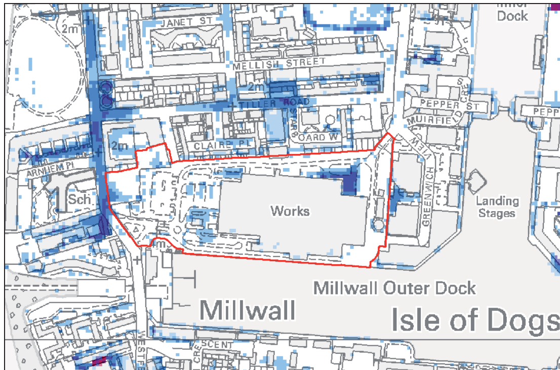
Figure 30-4 Maximum Depth of Surface Water in a 1% AEP Rainfall Event at the Westferry Printworks Site
