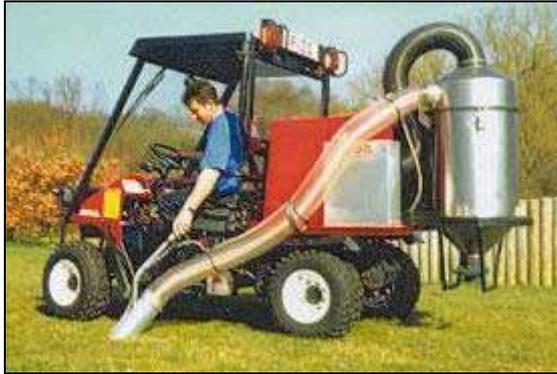
The collection unit contains its own engine, which drives a powerful vacuum unit capable of collecting 120 litres of all types of dog faeces. Once collected into a stainless steel container, it is mixed with disinfectant and water, which turns into slurry, leaving it pourable for disposal. A disinfectant spray pump is also fitted, not only to ease removal of stubborn faeces, but also to wash and disinfect the offending areas helping to protect children from toxocara canis.
