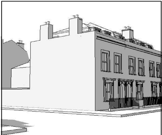
Mansard roof with inboard staircase
