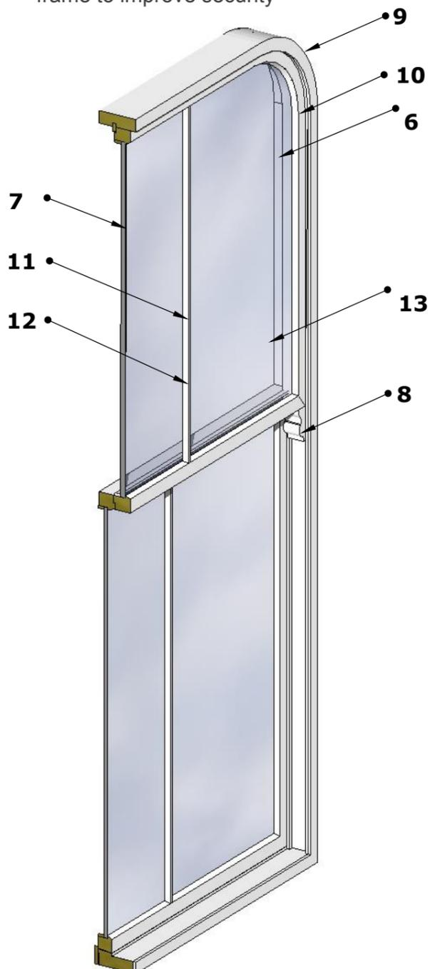
Typical timber sash window components
