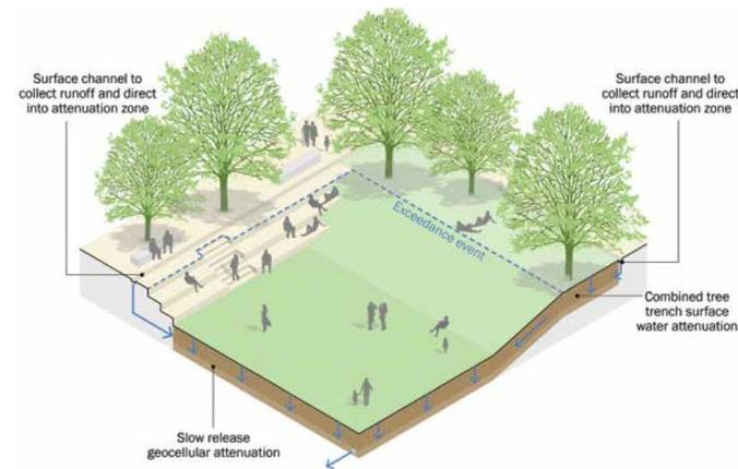
Figure 6-3 Example of Multi-functional civic space providing exceedance storage SuDS Manual C753
