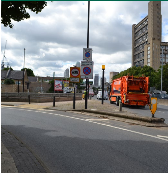
↑ Wide Abbot Road approach from the A12 encourages higher vehicle speeds, making north-south pedestrian movement unsafe
