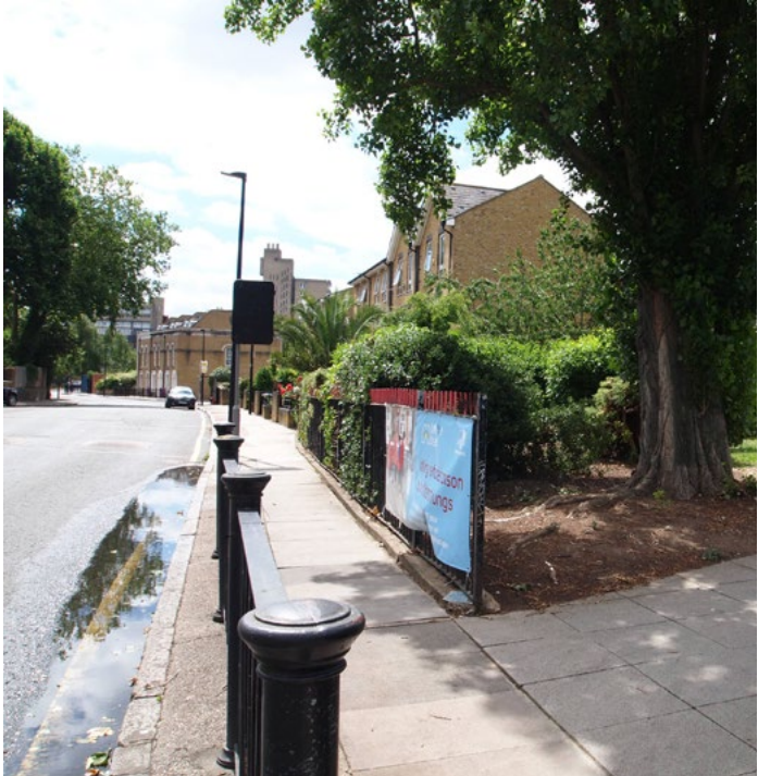
↑ Langdon Park diagonal path entrance by St Leonards Road - guard-railing and no dropped kerb restrict pedestrian and cycle movements
