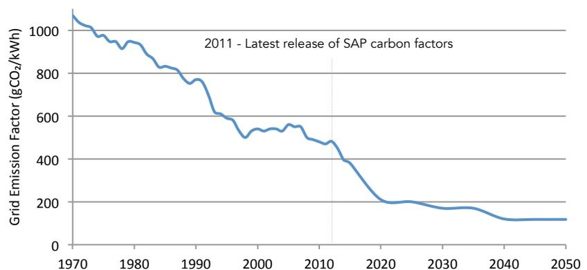
**Figure 4.09 - Past and projected future CO<sub>2</sub> emissions factors for grid electricity assumed in this study**
