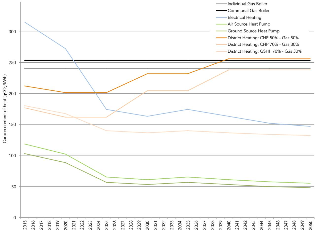
**Figure B.02 - Carbon content of heat from different heating technologies**
