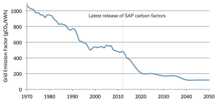
**Figure B.01 - Past and projected future CO<sub>2</sub>e emissions factors for grid electricity assumed in this study**
