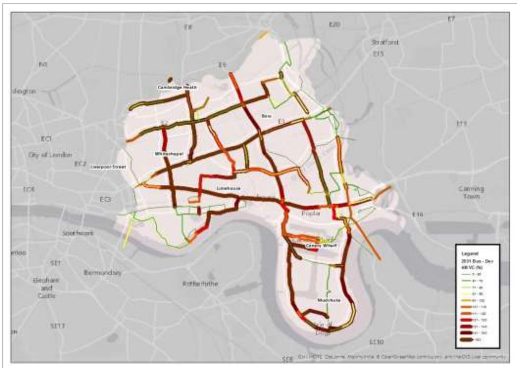
Figure 8.12 AM Peak Bus Patronage over Service Capacities (Mitigation Test 1, 2031)
