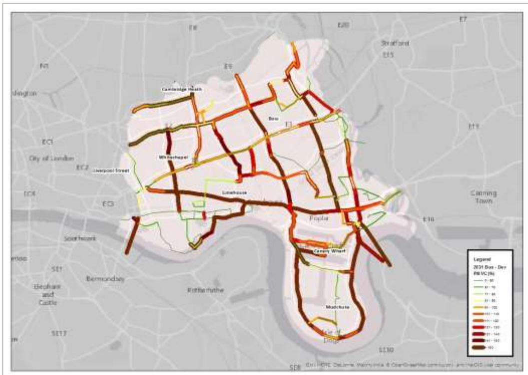
Figure 8.16 PM Peak Bus Patronage over Service Capacities (Mitigation Test 1, 2031)
