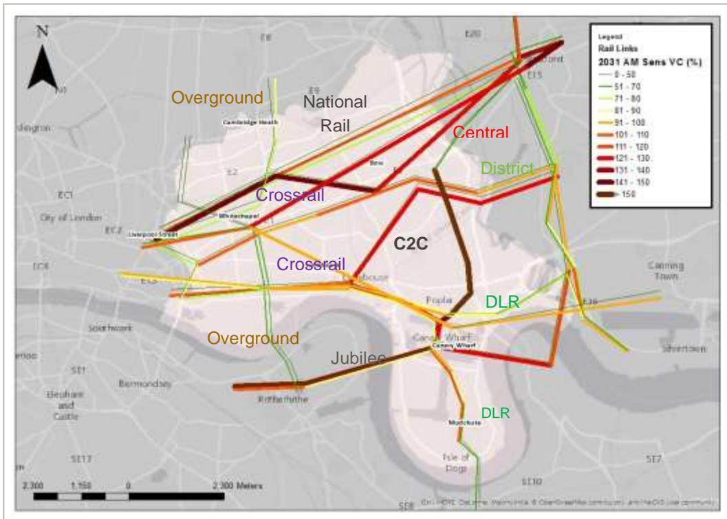
**Figure 8.4 AM Peak Rail Passenger Volume over Link Capacity (Mitigation Test 1, 2031)**
