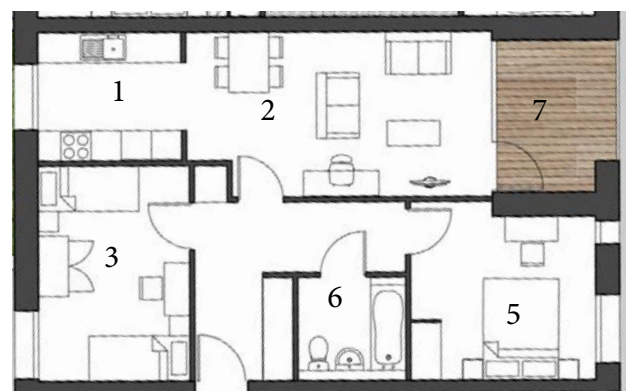
Example of dual-aspect floor plan including inset balcony (7); separation between kitchen (1) and living room (2) if needed, with possibility of cross ventilation through both; flexible twin room (5) which could also be used as a double bedroom; storage space integrated into plan. (image ©Levitt Bernstein)
