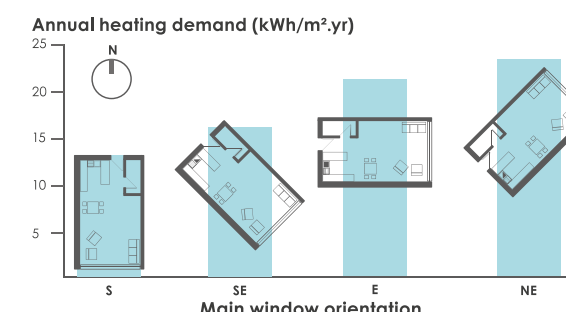
The diagram shows the impact on space heating demand as the same building is rotated. (diagram adapted from LETI).
